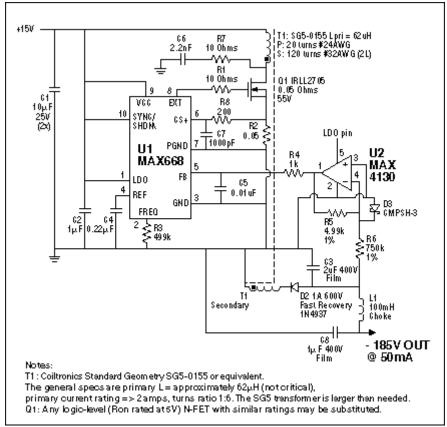
This circuit uses the MAX668 and a transformer (which will need about a one-to-six turns ratio) to make a flyback converter. The op amp inverts the feedback from the negative output voltage.
